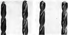
Modified drill (left) for cutting stainless steel has cutting edges beveled to give rounded effect, as contrast to sharply pointed edge of conventional drill (right).
